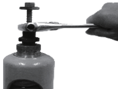
Fig. 8 Adjustment method of set pressure
